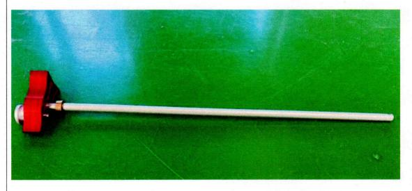
6. Assemble the optimized middle control box cover with the center console middle housing that has been repaired with the installation hole, then insert the handle and valve stem assembled in step 5 into the installation hole of middle control box cover and install them together on the aircraft. Finally install the throttle assembly and other fasteners, as shown in the following figure.
